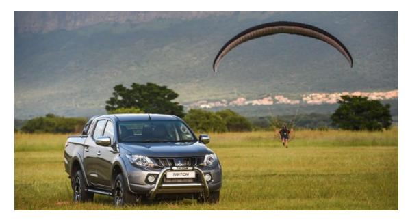
Gone are the rather bland looks, workman-like interior and 2.5 engine of the old generation and up steps a spruced up, well decorated and well-furnished bakkie armed with a much more sophisticated 2.4 turbodiesel engine that produces a solid 133kW and 430Nm from as low as 2 500rpm.
