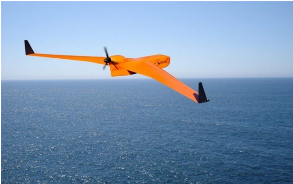
Boreal AJS 3 drone is used to take measurements at a very low altitude above the sea. boreal-uas.com
