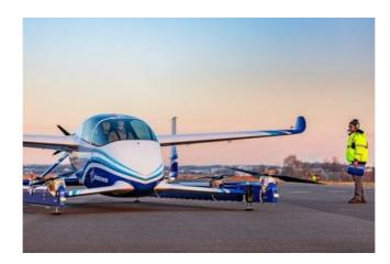
The PAV prototype completed a controlled takeoff, hover and landing during the flight, which tested the vehicle's autonomous functions and ground control systems. Future flights will test forward, wing-borne flight, as well as the transition phase between vertical and forward-flight modes. This transition phase is typically the most significant engineering challenge for any high-speed VTOL aircraft.
